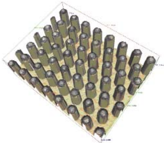
Figure 1. A 3D Copper Impregnated Micro HeX Plate model, measuring 700 \mu\text{m} x 550 \mu\text{m} x 150 \mu\text{m} high
