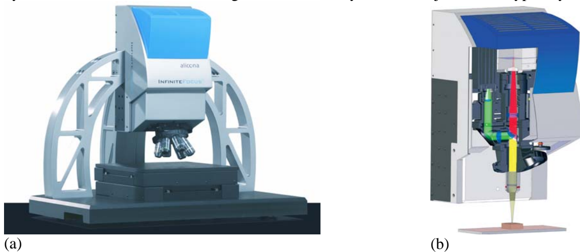
Fig. 1: (a) IFM G4 laboratory system (b) schematic visualization of the focus-variation technology. The small depth of focus of the optical system is used to extract depth information with registered true color.
