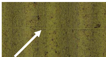
Fig. 2: An optical color image of a sinusoidal roughness standard ( R_a = 500\text{nm} ) obtained by the InfiniteFocus device. The image shows the horizontal trace of a contact stylus instrument that has been used for reference roughness measurements.
