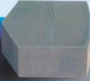
Micro- contour-artefact, calibrated by PTB
