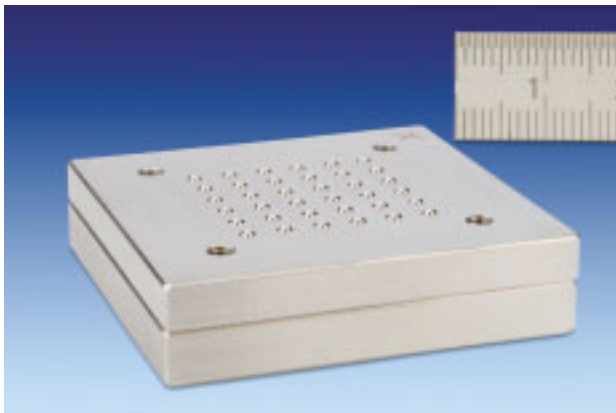
Ball plate with 6 x 6 steel balls, radius 1 mm, distance 4 mm, smooth surface, balls clamped from bottom side
